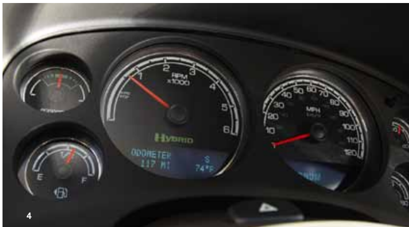
↓ Yukon Denali Hybrid's analog gauge cluster keeps you up to date and in control of your vehicle's speed, mileage, fuel levels and more.
