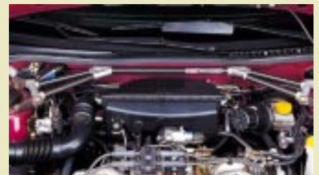
Strut tower brace-carbon fiber. Carbon fiber and high-strength aluminum construction effectively distributes stress loads via three bolt strut-top mounts.
