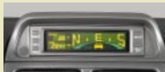
Gauge pack. Displays compass, outside temperature and barometer or altimeter readings.
