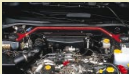
Strut tower brace-steel. Provides additional stiffness to the upper suspension area. Reduces strut deflection to promote quicker steering response.
